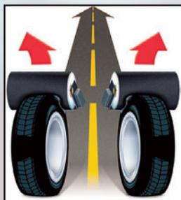
identifies lateral forces. Again the large roller is utilised to measure the amount and direction of pull of each tyre. Tyre assemblies are tagged for identification purposes. When the measurement of either a pair or all four wheels is complete a recommended best position for each wheel is suggested. The aim is not to reject any one tyre but to balance tyres across an axle (particularly the front axle) relative to one another, on the vehicle to obtain the best straight-ahead steering stability.
