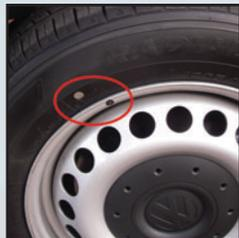
Tyre uniformity is measured in assembly plants and manufacturing facilities, and wheel tyre assemblies have been matched to ensure the smoothest of ride for that new vehicle feel.
